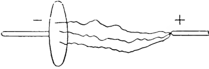
FIG. 10.—Connections of the X-Ray tube to the coil (Schall), showing the route travelled by the sparks when the point is the positive pole and the negative the plate.
